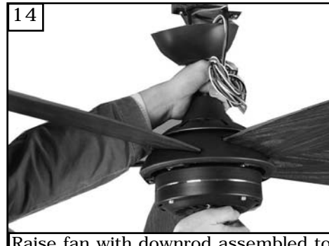
14 Raise fan with downrod assembled to the ceiling bracket and hang fan assembly. Be sure to rotate the downrod ball so that the notch in the bracket engages the slot in the ball.
